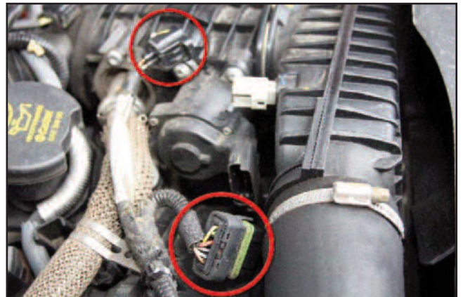
Butterfly valve connector (lower) and air box connector (upper)
