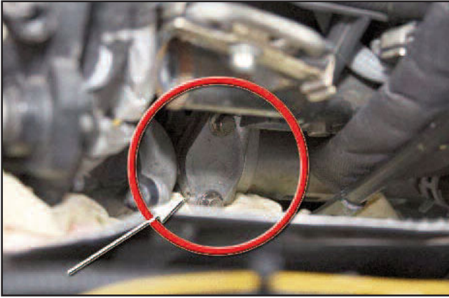
EGR valve blank fitted – indent arrowed!
