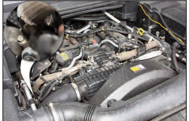
View of engine with top cover removed – right hand EGR valve shown in inset
